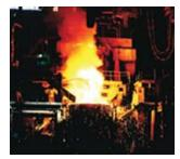
Upon achieving the desired chemical composition, molten metal is poured into Ladle. Purging is done to the molten metal tapped to the ladle to achieve homogenous chemistry and temperature throughout the ladle. In order to avoid thermal stratification that leads to undesirable varying steel compositions, nitrogen gas purging is done. Purging is conducted by generating bath turbulence to retain thermal homogeneity. This process also helps in removing excessive non-metallic inclusions
