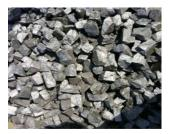
Ferro Alloys are added for refining the molten metal to achieve the desired level of chemical composition. The molten metal is fully killed by adding ferro alloys such as silico manganese, aluminum. Throughout the melting process and micro alloying elements addition process, samples are chemically analyzed to ensure accurate and desired chemical composition.
